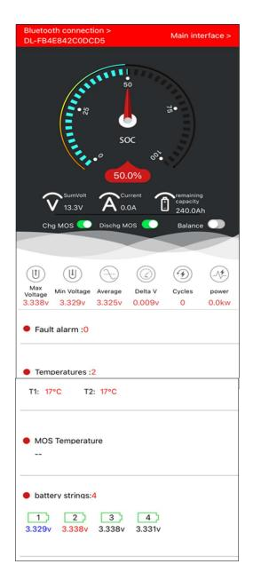
Look for the Bluetooth ID corresponding to the batteries. The Bluetooth ID is listed on the battery label, which can be found on the outside back cover of this manual and the outside back face of the battery case. Note that the vehicle has two batteries, and each has it's unique Bluetooth ID.
