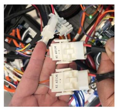
2-wire connection of DC emergency charge cable in the electrical compartment
