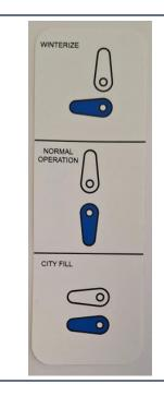
Winterize – This uses the pump to draw Winterizing fluid into the pump and add it to the tank.
