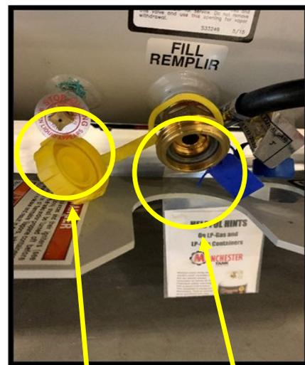
Propane bleed valve (left) and Fill valve (right)
